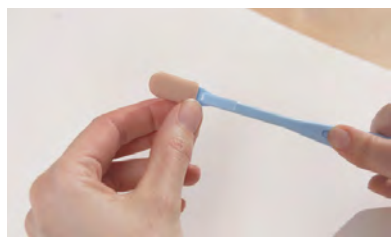
Gently pull Sofft Cover completely over Knife tip (like a sock). Covers can be re-used several times.
